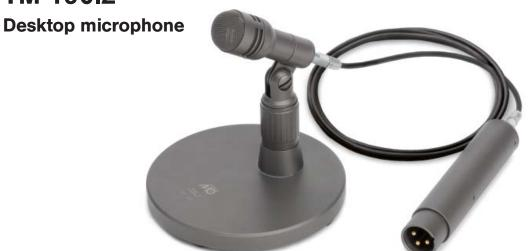
The TM 190.2 desktop microphone is a compact version of Studio condenser microphones series micon. It is specially designed for commentary, translators and applications in TV and Radio. It is a classic 48V phantom powered condenser microphone design, which ensures a high degree of speech intelligibility even in unfavourable acoustic conditions. Its unobstructive appearance also makes it ideal for use on conference tables.
